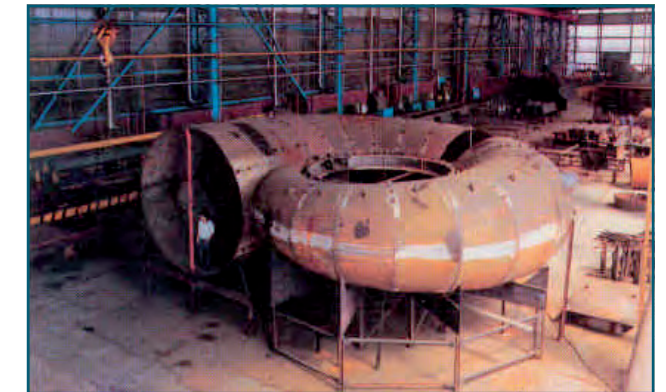
A spiral case in the sheet metal shop Dadin Kowa project, Niger
