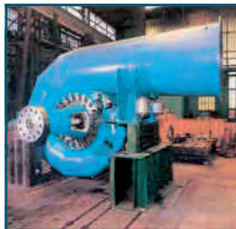
Fig. 1. The cooling system of several thermal power stations were installed with our recuperative Kaplan turbines. The machines on the picture were delivered to Trakya project in Turkey
