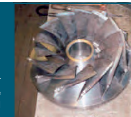
Welded runner for Barnes Bridge project, England
